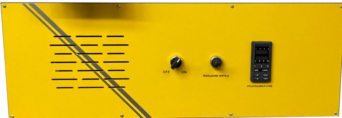
Temperature and cooking cycle control is entrusted to a Lumel RE82 microprocessor programmer. A maximum of 15 programs can be configured and stored, each consisting of a maximum of 15 ramps.
