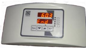
Temperature and firing cycle are managed by a microprocessor programmer mod. K1PX, with which it is possible to memorize 4 firing cycles, each consisting of 8 steps.
