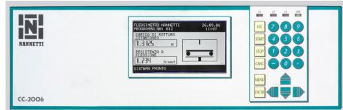
The management of the test is entrusted to an electronic control unit, which will give the final result, as a module of rupture, expressed both in Newton/mm<sup>2</sup> and in Kg/cm<sup>2</sup> and as breaking load expressed both in Newton and in Kg.
