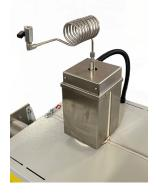
The working tube forming the furnace chamber is equipped with a chimney, which can be heated up to a maximum operating temperature of 300 °C, through which the gases that form inside the furnace can pass and can be conveyed to other instruments for analysis.
