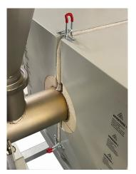
The construction of the furnace body is made of two horizontally opening parts, mounted on slides to allow quick and easy maintenance, replacement of heating elements and possible replacement of worn parts
