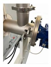
This kiln is designed to work even in a controlled atmosphere; there are four inert gas clutches, two at the inlet and two at the outlet.
