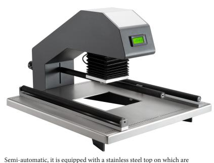
positioned two supports (knives), moved and adjusted manually and individually, which receive the sample to be tested.
