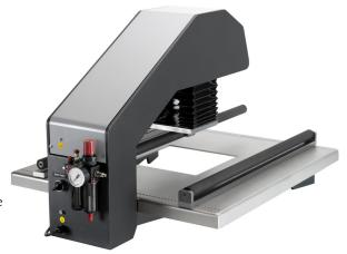
The management of the test is assigned to an electronic control unit which will give the final result expressed both in Newton/mm $^2$  and in Kg/cm $^2$  and the force exerted to break the tile both in Newton and in kilograms.
